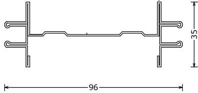
273019000 Teleblind S 1195 Telelux blind 1195mm | Teleblind cross-piece 1195mm Teleblind Zwischenprofil 1195mm L=1195mm
